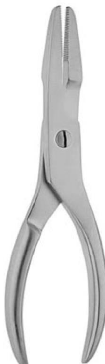
7-420 Wire Bending Cutting Pliers soft wire 1.5 mm hard wire 1.0 mm
